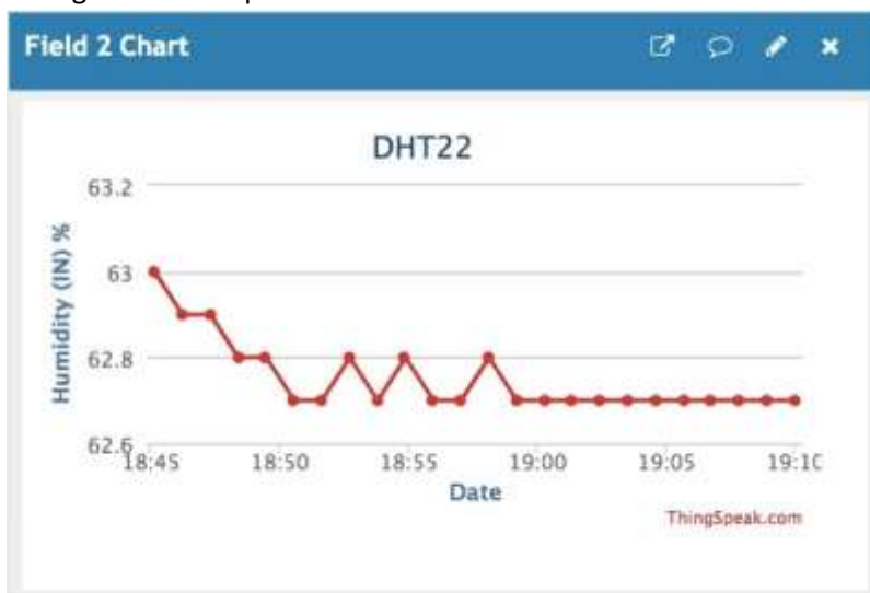
Figure 51: Humidity monitored inside the chamber
